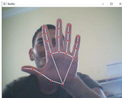
Figure 12. Detection and counting of fingers from the image
