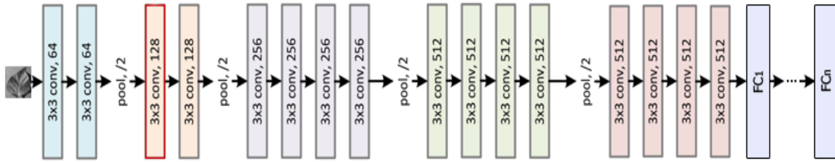
Figure 2. VGG-19 architecture and fine-tuning process in dense layers
