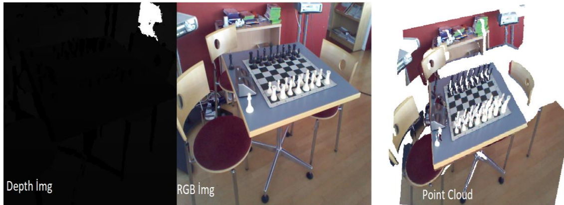
Figure 2. RGB-D image to point cloud
